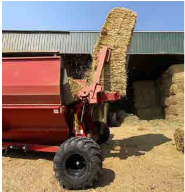
Figure 5.22: Second Bale Loaded on Bale Lift
