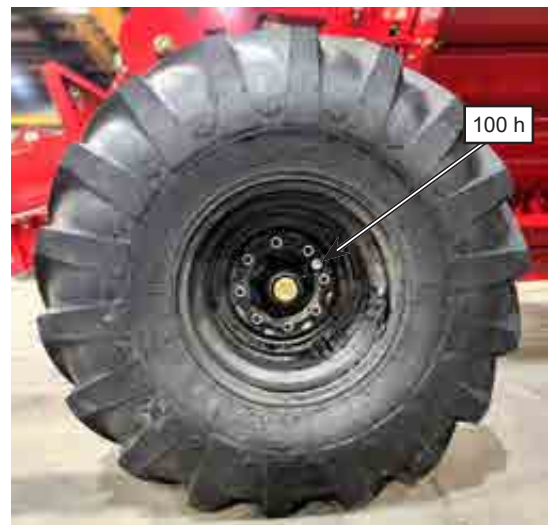
Figure 6.5: Grease Hubs on Spindles
