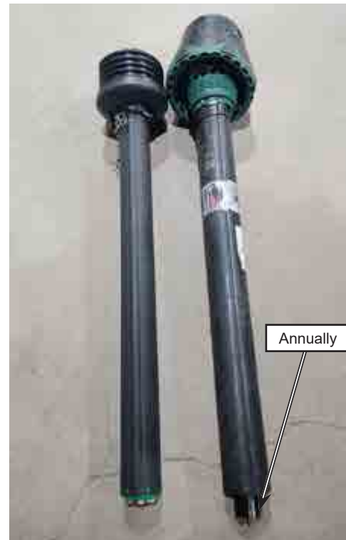
Figure 6.7: Grease the Sliding Portion of the Drive Shaft
