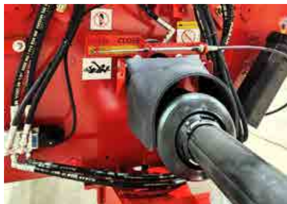
Figure 4.26: Ensure Drive Shaft Shield is in Place
