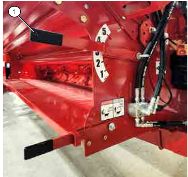
Figure 5.8: Set the Aggression of the Flails
