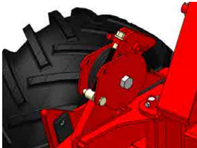
Figure 6.28: Relieve the Spring Tension
