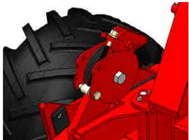
Figure 6.32: Install the Tension Bolt and Bar
