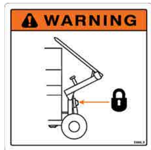
15 - Warning - Install Cylinder Lock Before Going Under Raised Bale Lift
