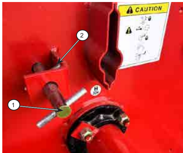
Figure 4.37: Remove the Flail Drum Lock
