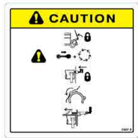
18 - Caution - Shut Down Tractor and Lock Bale Lift and Flail Drum Before Using Twine Cutter
