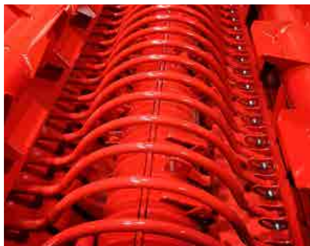
Figure 4.33: Move Flails Blocking the Knife Path
