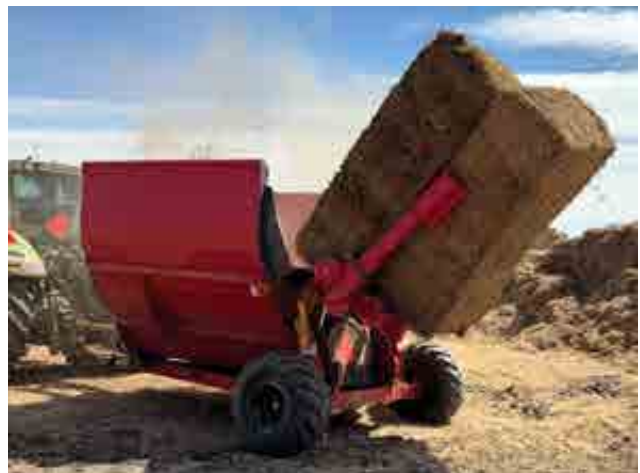
Figure 5.23: 2 Bales Loaded on Bale Lift
