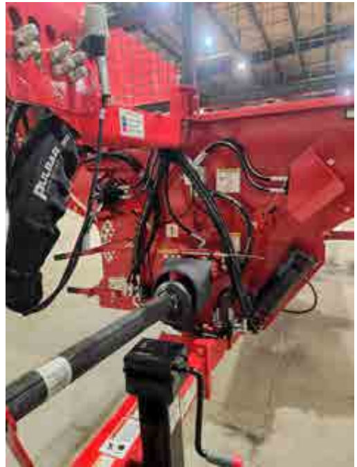
Figure 7.8: Hoses and Electrical Connectors Secured
