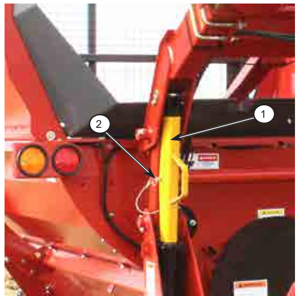
Figure 4.11: Lift Cylinder Locked
