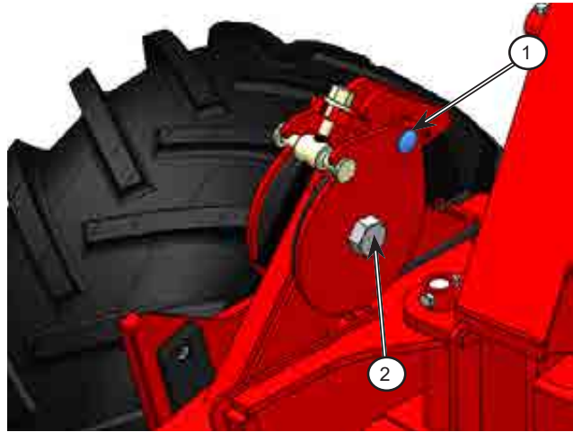
Figure 6.33: Install the Locking Bolt
