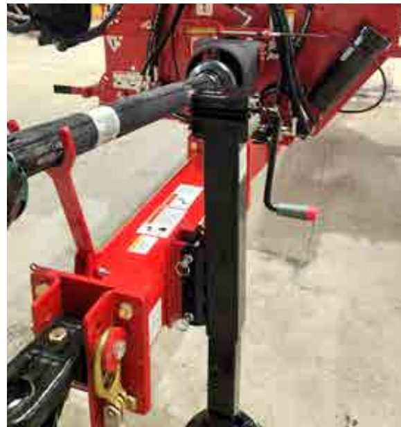
Figure 4.3: Lift Hitch with the Jack
