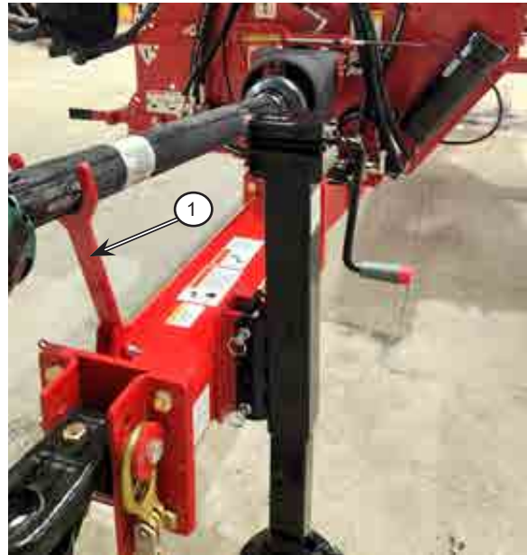
Figure 7.6: Lift Hitch with the Jack
