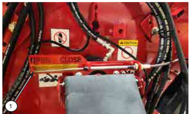
Figure 5.19: Clamping Arm Position Indicator
