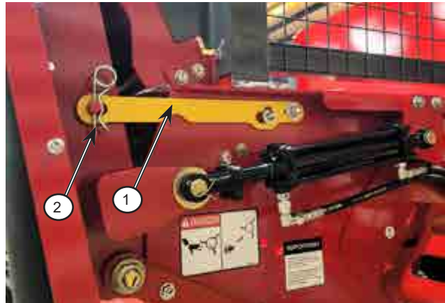
Figure 5.11: Discharge Door Lock
