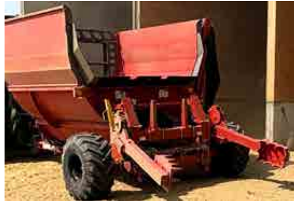
Figure 7.2: Bale Lift Lowered
