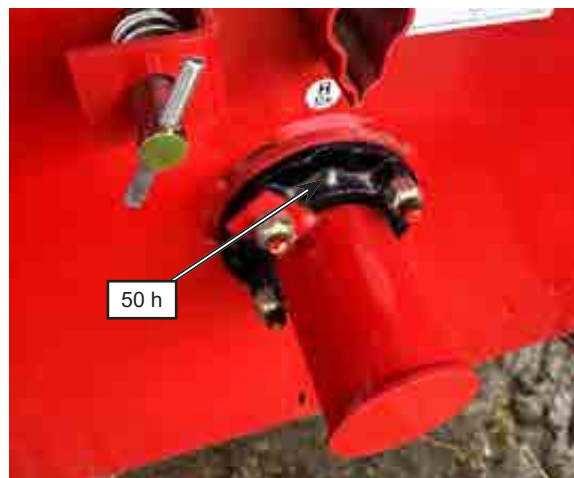
Figure 6.2: Grease Rear Flail Drum Bearing
