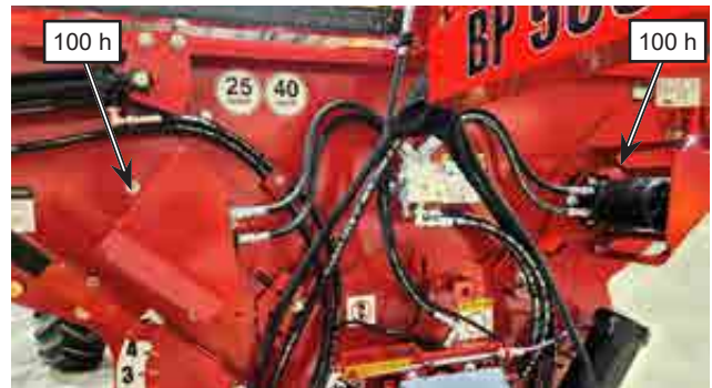
Figure 6.3: Grease Front Feed Roller Bearings
