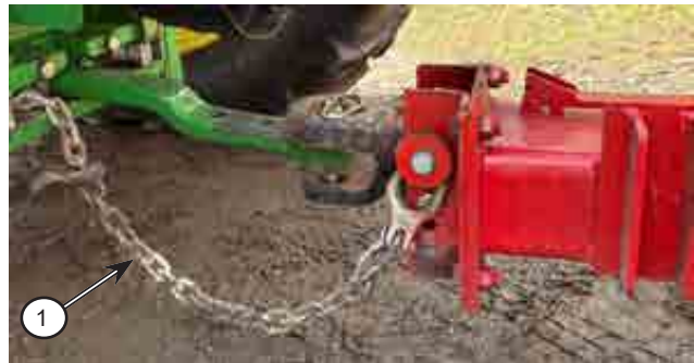
Figure 7.7: Disconnect the Safety Chain
