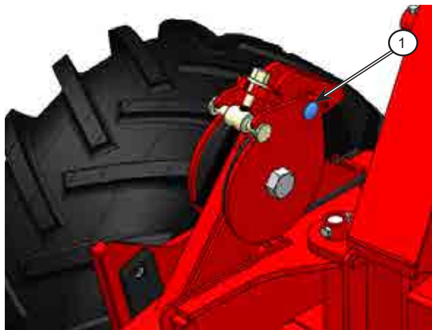
Figure 6.27: Tension until Locking Bolt is Loose
