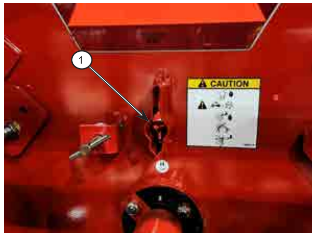
Figure 4.36: Insert Twine/Wrap Cutter into the Guide
