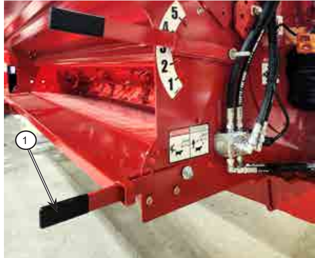
Figure 5.16: Set the Lower Discharge Deflector
