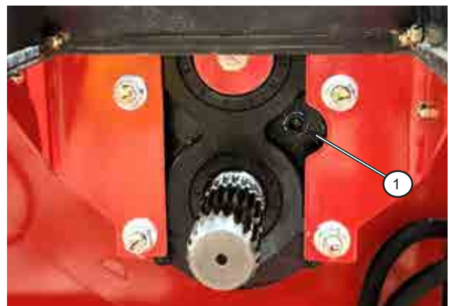
Figure 6.12: Check Gearbox Oil Level (Drive shaft shown removed for clarity)
