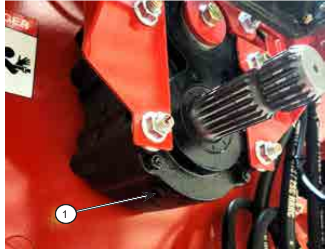
Figure 6.10: Drain Oil from Gearbox (Drive shaft shown removed for clarity)
