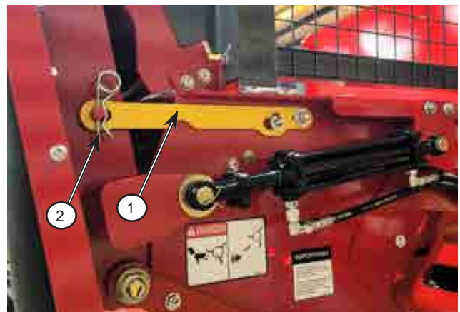
Figure 7.5: Discharge Door Lock
