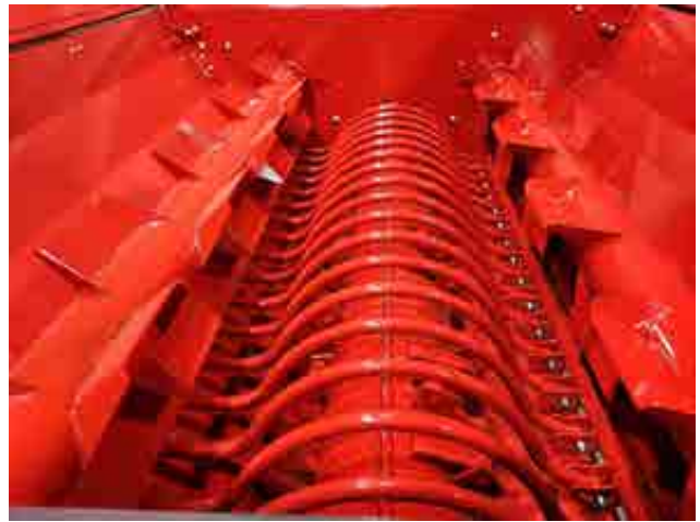
Figure 4.40: Remove Wrap/Twine from Feed Rollers
