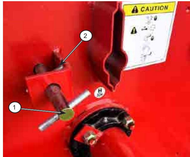
Figure 5.1: Remove the Flail Drum Lock
