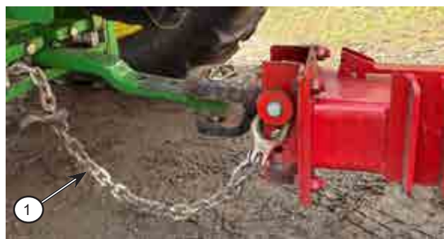
Figure 4.5: Connect to the Tractor Drawbar and Connect the Safety Chain
