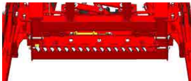
Figure 4.20: Check that the Twine Sickle™ Moves
