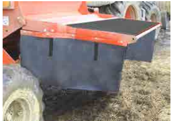
Figure 5.13: Rubber on Top of Door for Bedding
