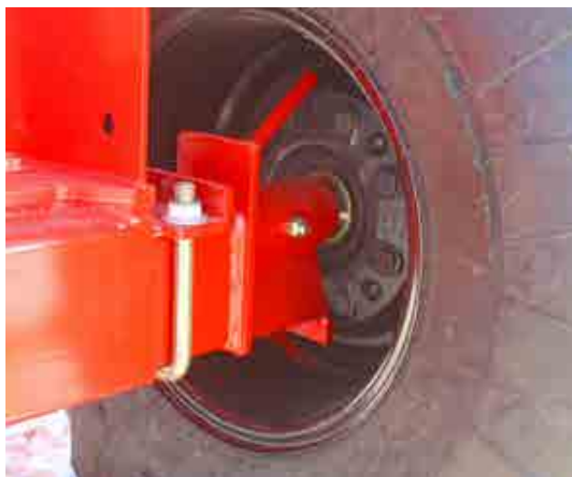
Figure 6.22: Remove Twine/Wrap from Spindle & Hub
