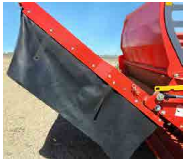
Figure 5.14: Side Curtains Loosened for Bunk or Windrow Feeding
