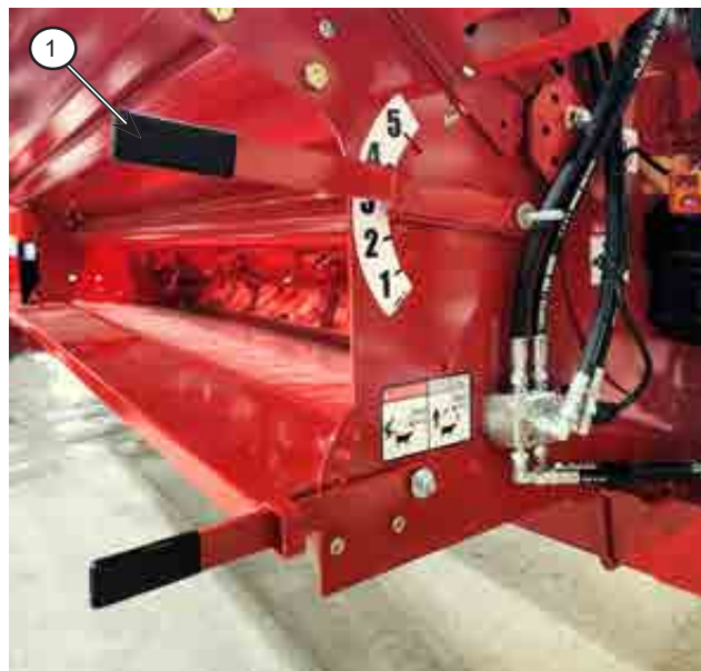
Figure 4.31: Move Flail Guard Rod Lever
