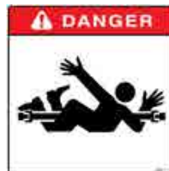
Figure 4.26: Ensure Drive Shaft Shield is in Place
