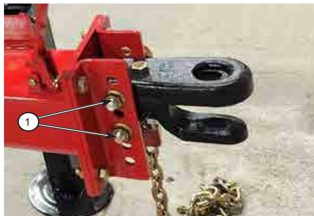
Figure 4.4: Adjust the Hitch Tongue
