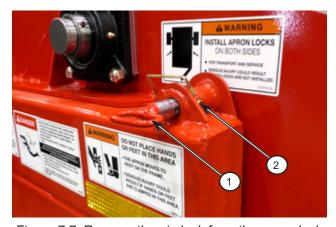
Figure 7.7: Remove the pin lock from the apron lock
