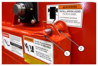
Figure 6.6: Remove the locking pins
