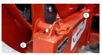
Figure 7.8: Install the apron lock
