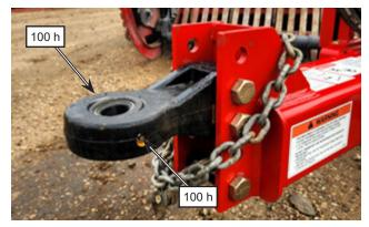
Figure 6.18: Grease hitch tongue
