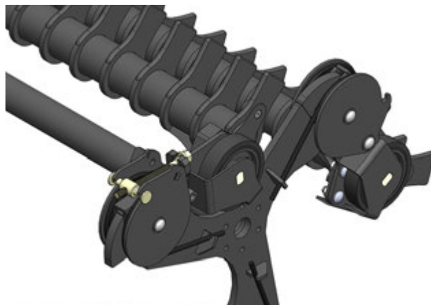
Figure 6.37: Relieve the spring tension (Only reel shown for clarity)
