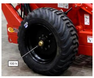
Figure 6.17: Grease wheel hubs
