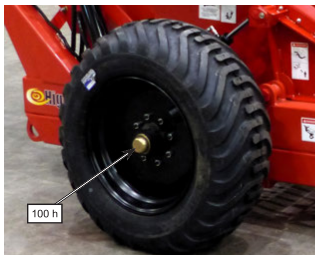
Figure 6.17: Grease wheel hubs
