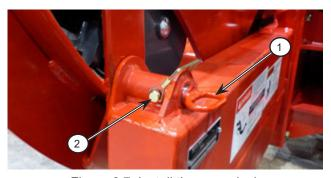
Figure 6.7: Install the apron lock
