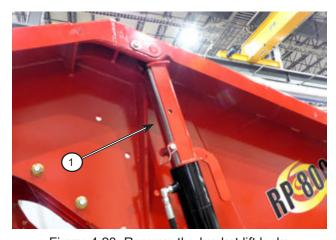
Figure 4.23: Remove the bucket lift locks
