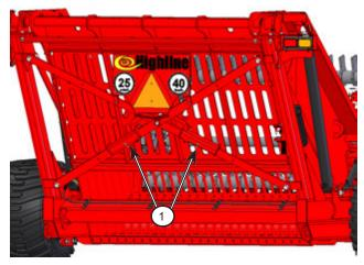
Figure 4.18: Remove the bucket lift locks from the storage position
