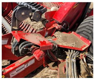
Figure 4.16: Remove debris from the frame
