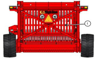
Figure 4.27: Rear bucket dump height panel
