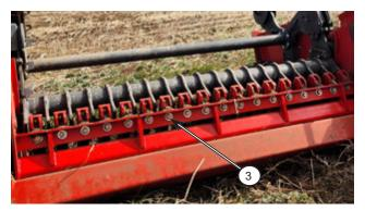
Figure 6.27: Check the bolts on each tine
