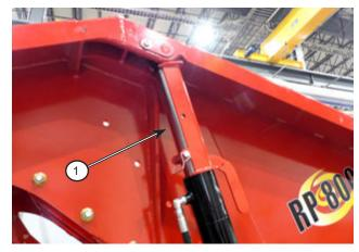
Figure 4.19: Install the bucket lift locks
