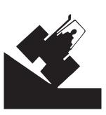
13. Do not operate tractor and implement(s) close to a ditch or embankment. An unstable bank will give way causing a side overturn. Operate at least as far from the edge of a ditch as that ditch is deep.
