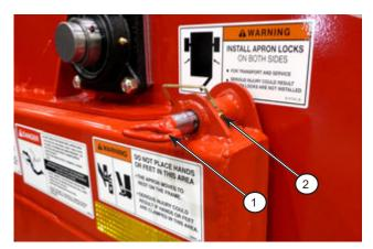
Figure 6.9: Place apron lock in storage position
