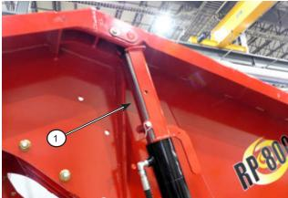
Figure 6.3: Remove the bucket lift locks
