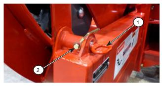
Figure 4.8: Install the apron lock
