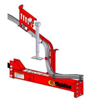
Figure 4.4: Place the jack in the storage location
