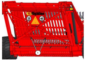
Figure 6.4: Place bucket lift locks in storage position
