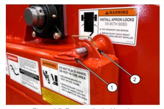
Figure 4.7: Remove the locking pin
