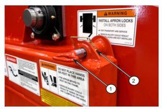
Figure 7.2: Place apron lock in storage position
