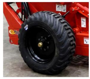
Figure 6.23: Check tires and adjust air pressure
