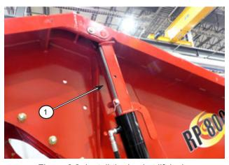
Figure 6.2: Install the bucket lift locks
