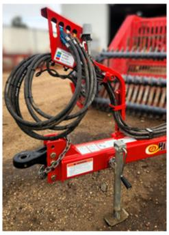
Figure 7.10: Secure the hydraulic hoses and electrical connections to the hose holder
