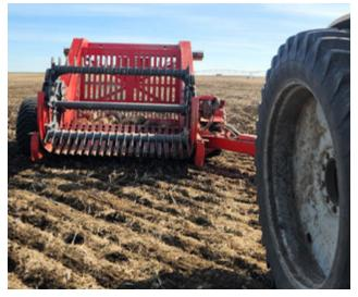
Figure 5.8: Rock Picker in working position
